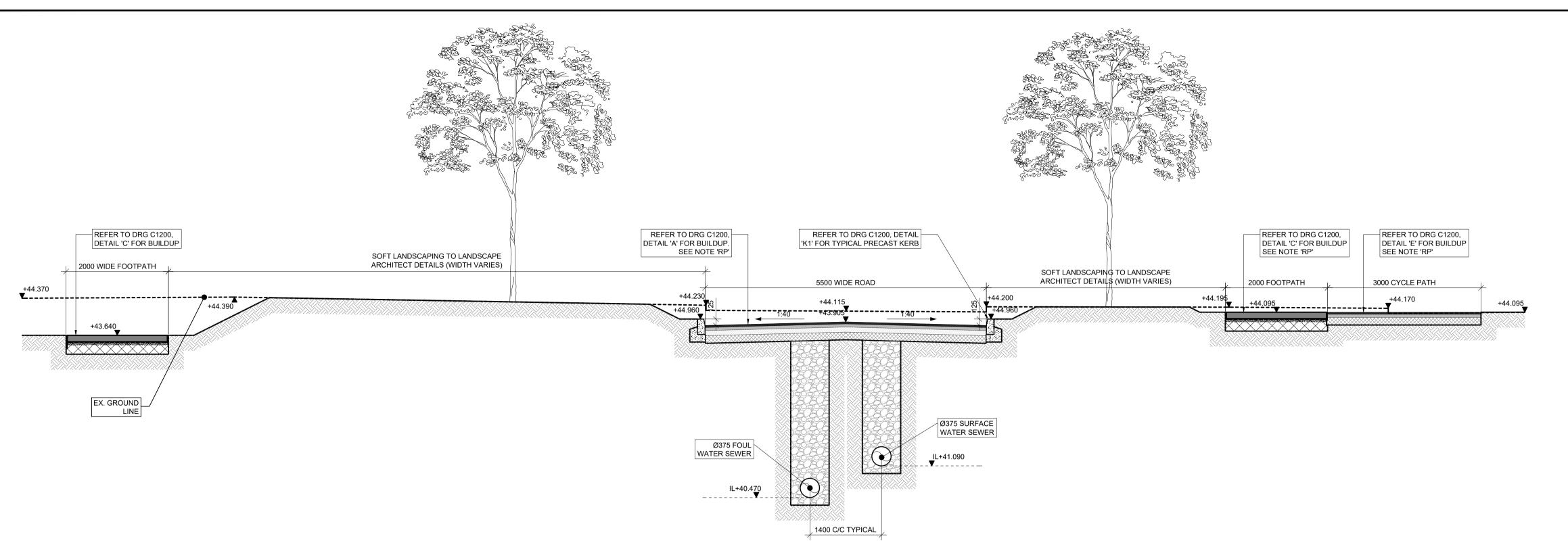
TYPICAL DETAILED CROSS SECTION THROUGH AVENUE LEADING FROM THE NORTH ACCESS TO THE DUNDRUM ROAD NORTH ACCESS (DRAINAGE SHOWN)
